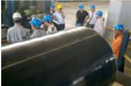
A view of the 30 inch steel pipe coated and tested at the Petrojet factory at Port Said, Egypt
